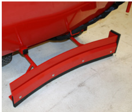
Rubber on scraper can be replaced.
