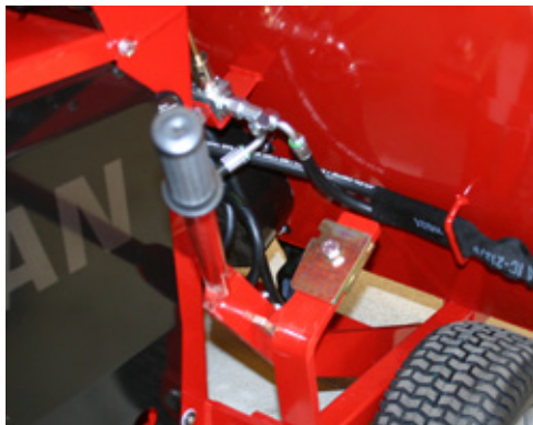
Adjustment of scraper height using 19 mm spanner
