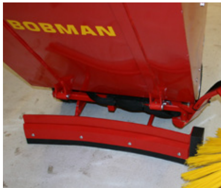
Rubber on scraper can be replaced.
