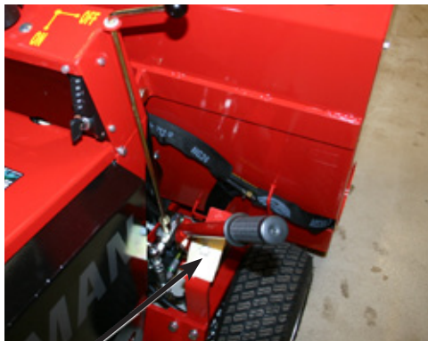
Adjustment of scraper height using 19 mm spanner
